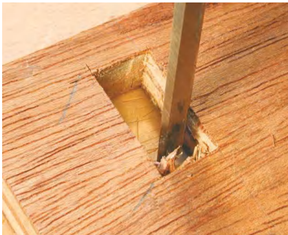
▲ Pic.1 A chisel needs to have very sharp edges for accurate paring
